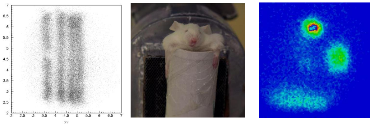
Planar images of simple geometrical phantoms and specific organs of a small mouse using ^{99m}\text{Tc} radiotracer.
